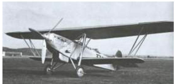
Fokker CV-E-1, 860 PS, 318 km/h, 10.8 m/s
