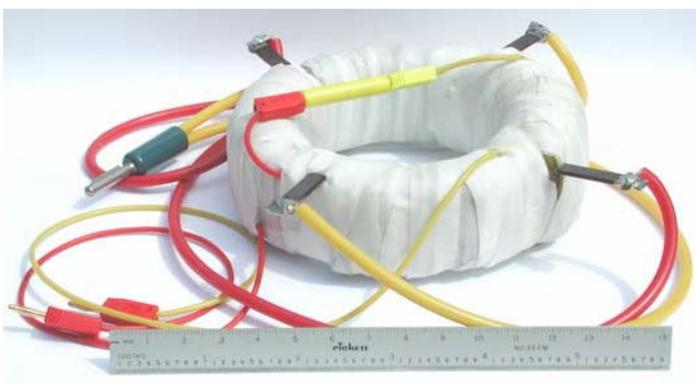
An experiment with the new pulse transformer in the photo, built with a modern tape-wound toroidal core of high saturation flux density and low eddy current loss, has confirmed that the power requirements of the modulator can be met with a reduced stored electric energy of only 0.32 joules. For the reduction of the leakage inductance a subdivided winding configuration is employed.
