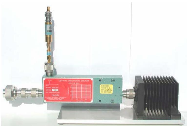
For the RF peak power measurements the Hohentwiel-transmitter was operated through a Narda directional coupler into a dummy load. The power was measured with a Boonton Electronics peak-power sensor model 56318, at the directional coupler and indicated on the Boonton Electronics model 4530A peak-power meter. The pulse shape could be observed either on the display of the 4530A or with the HP8472A detector.
