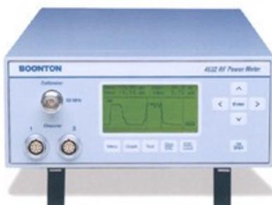
The Boonton Electronics 4530A Peak Power Meter in combination with the 57318 Peak Power Sensor, allows peak power measurements between +20 to -39 dBm with an accuracy of  $\pm 0.06$  dB (2.1%).
