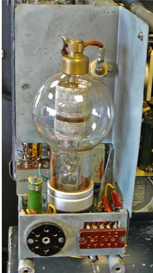
**Original FuG 200 inductive transmitter coupling loop**
