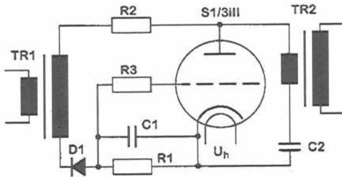
A simplified functional diagram of the thyatron modulator appears on the left. At the end of the charge cycle the capacitor C2 stores an electrical energy of 0.7 joules at 800 volts.
