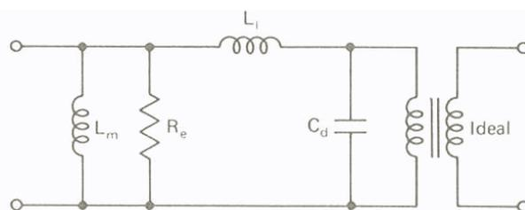
The pulse transformer TR2 is the most critical component of the Hohentwiel modulator. Its development was a trade-off between conflicting requirements. The figure shows the simplified equivalent circuit for a pulse transformer.
