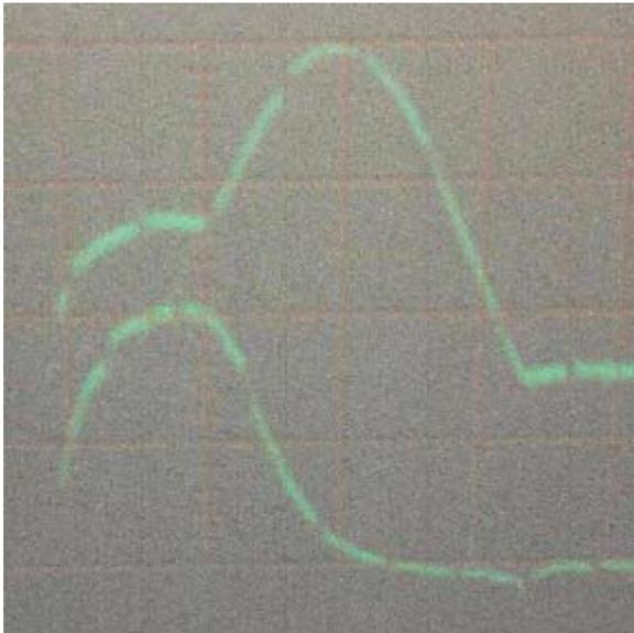
Upper Trace: Primary current of the pulse transformer during the discharge of 0.7 joules stored in capacitor C2.
