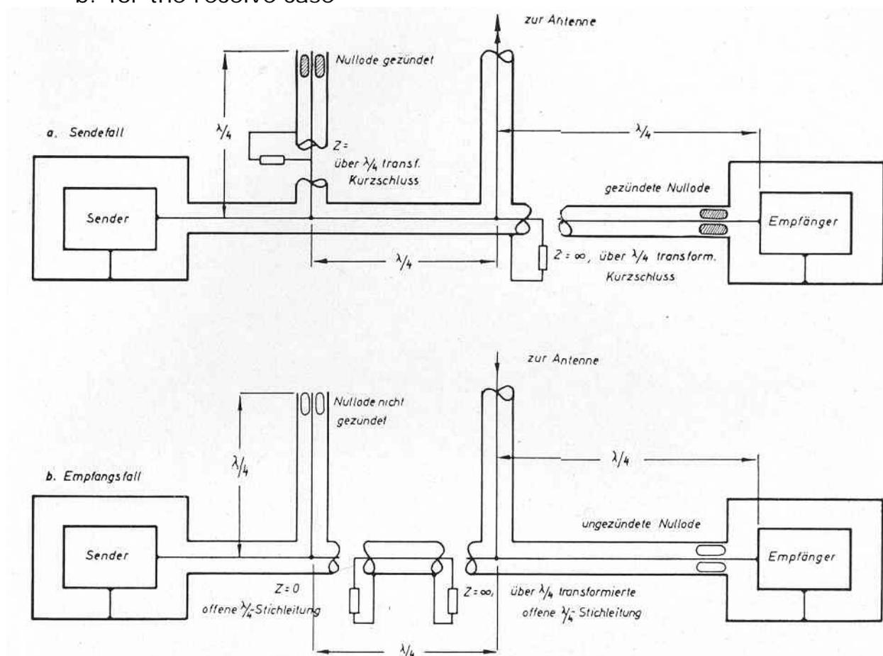
Gas-discharge tubes (German designation Nulloden) were utilized for the T/R switch device. The strong electric fields rapidly ionize the gas, thereby presenting a very low impedance to the transmitted signal during the transmitted pulse.
