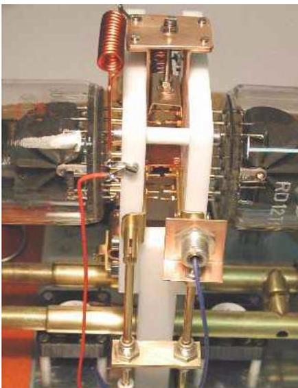
The power measurements were done at 525 MHz with a plate pulse voltage of approximately 9 kV.
