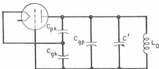
Grid-return oscillators can be made in which almost the only coupling between the frequency-determining plate circuit and the feedback to the cathode circuit is produced in the capacitive voltage divider formed by the internal tube capacities  $C_{pk}$  (plate-cathode 1.35 - 1.65 pf ) and  $C_{gk}$  (grid-cathode 6.3 - 7.7pf for the RD12Tf triode).
