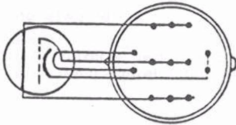
At left, the socket outline and electrical schematic of the RD12Tf tube. The construction of the tube system and the arrangement of the pins made it easy to employ symmetric Lecher line resonant circuits in push-pull oscillators.
