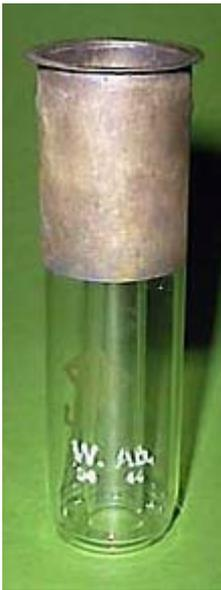
The figure on the left shows a photo of the Telefunken LG 71 TR-tube utilized in the Hohentwiel-Simultangerät as switch device (in Germany was the tube designated as a so called Nullode)
