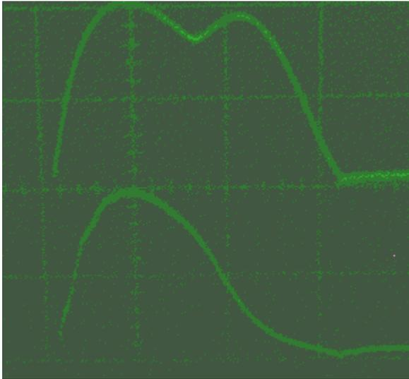
Upper Trace: Primary current of the new pulse transformer during the discharge of 0.32 joules electric energy.
