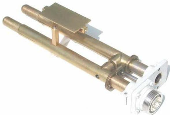
The photo shows the output circuit of the Hohentwiel - transmitter with the inductive coupling loop and the tuneable balun transformer. With the adjustable stubs of the Lecher lines shown at the left of the photo the output circuit is tuned to resonance with the transmitter frequency. The adjustable slide bar at the right enables to match the transmitter output to the load impedance.
