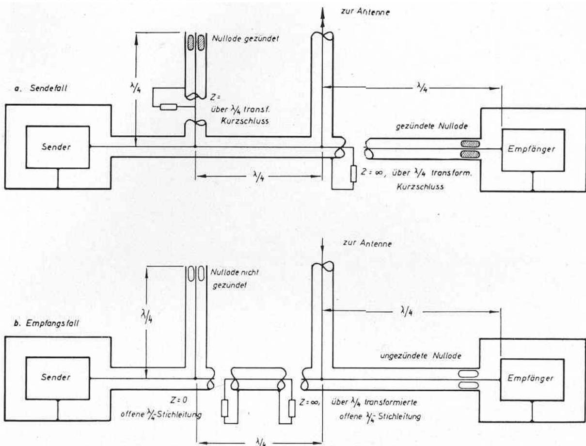
Gas-discharge tubes (German designation Nulloden) were utilized for the T/R switch device. The strong electric fields rapidly ionize the gas, thereby presenting a very low impedance to the transmitted signal during the transmitted pulse.
